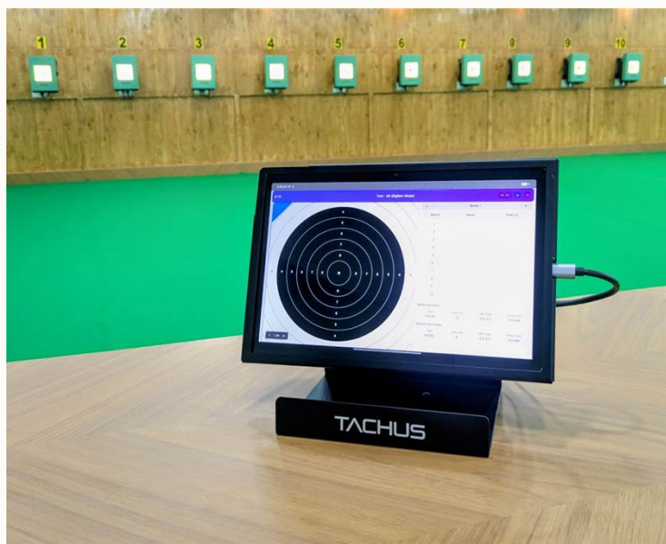
Scoring monitor with ten Tachus 10 ETS units downrange Fig. 01
